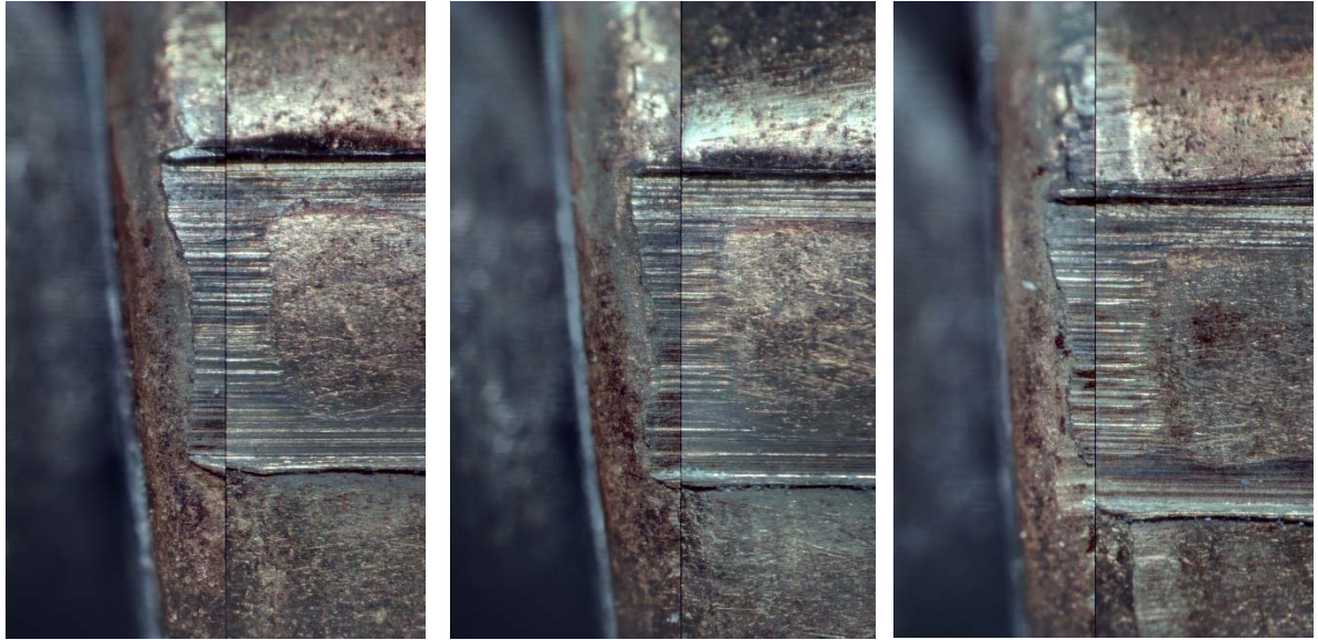
Figure 6: Three different land-engraved areas of TF-02-B and UNK-14 using VisionX
